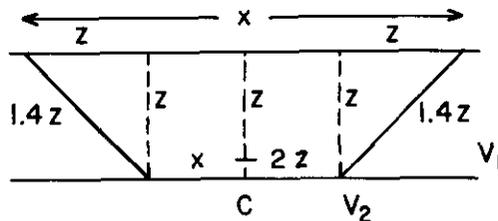
$$\text{Depth} = \frac{V_1 \left( T - \frac{x}{V_2} \right)}{2 \cos i}$$
