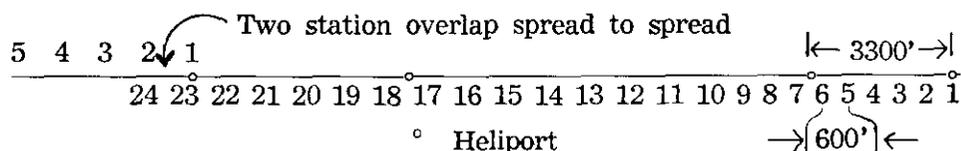
For each spread involving five heliports, two linemen were dropped into each of the three middle heliports, one into each of the two outside heliports. Each of the men layed out three stations and they met in pairs between the heliports. Communication was maintained with the recorder through a telephone line incorporated in the cable. The linemen carried hand phone units.
