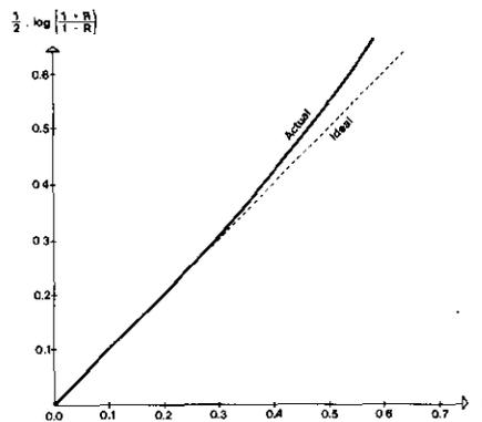
Fig. 1b. Curve of reflection coefficient,  $R$ , versus its logarithmic approximation.
