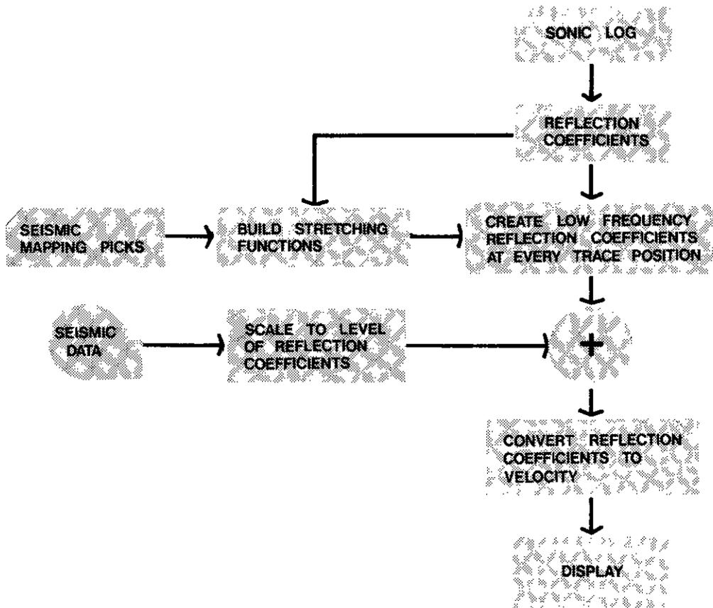
Fig. 8. Flowchart depicting a method of seismic inversion.
