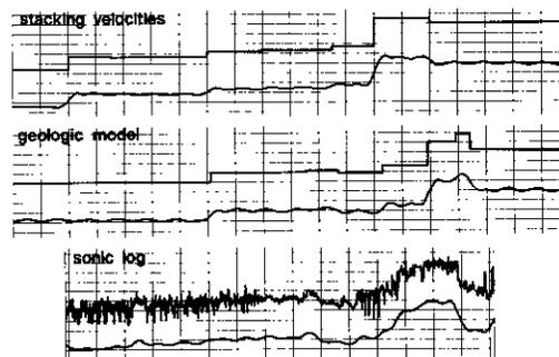
Fig. 5. Three possible candidates for supplying low frequency velocity information.
