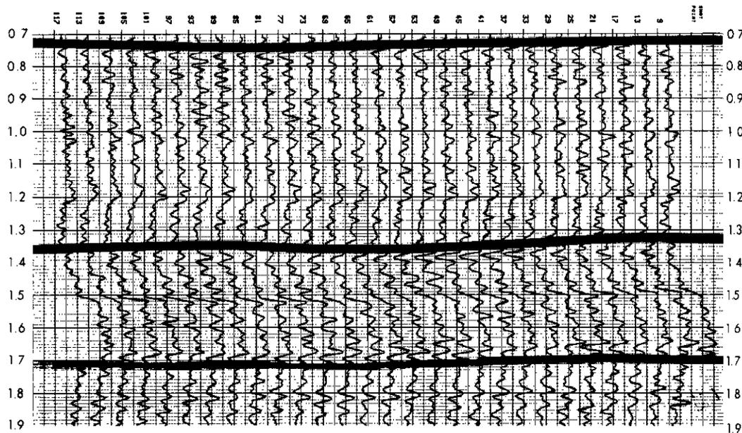
**Fig. 10.** Pseudo acoustic impedance logs derived by combining information in Figure 4 with that of Figure 9. Two events are picked at about 1.3 and 1.7 seconds for comparison with Figure 3.
