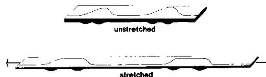
Fig. 6. Stretching a rubber sheet of uneven thickness — and the effect on a curve drawn on the surface.
