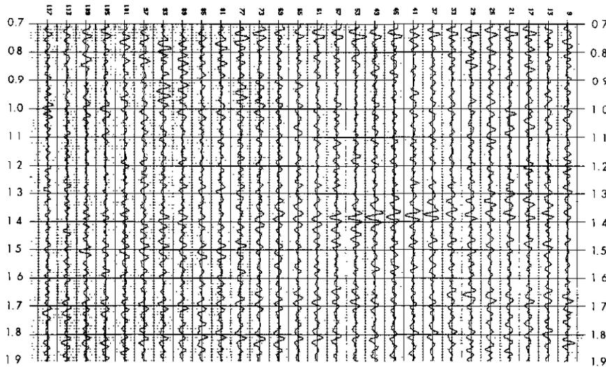
Fig. 4. Pseudo acoustic impedance logs derived from seismic section in Figure 3, using no low frequency information.
