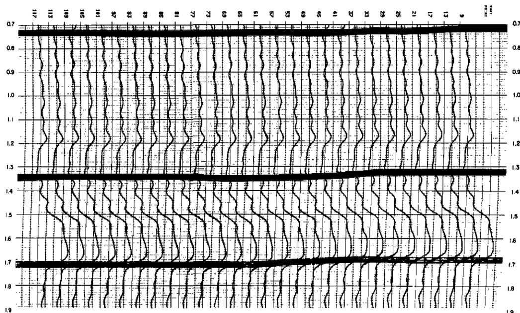
Fig. 9. Pseudo acoustic impedance logs derived from low-frequency velocity information only.
