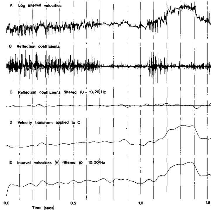
Fig. 2. Effect of mixing the use of filters and velocity transforms.
