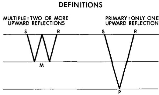
Fig. 1. Definition of Multiple and Primary Reflections.
