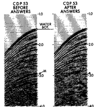
Fig. 14. Offshore Labrador 48 fold CDP Gathers — Deep Water.
