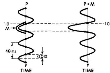
Fig. 4. Multiple and Primary Energy is Additive.
