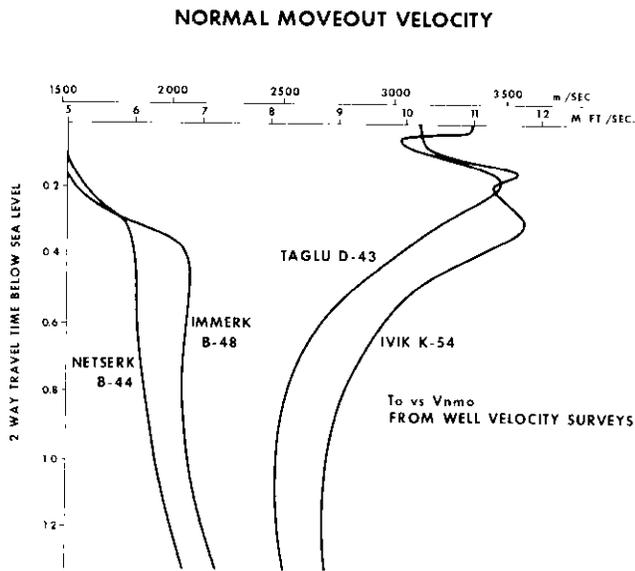
Fig. 8. T<sub>0</sub> vs V<sub>NMO</sub> from well velocity surveys.
