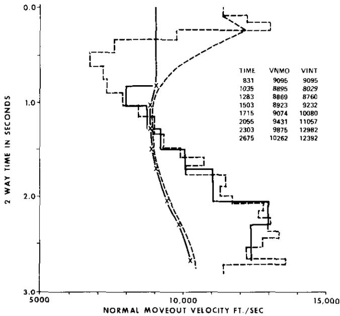
Fig. 10. Comparison of curves in Figure 9 with  $T_0$ - $V_{NMO}$  and interval velocity curves from a nearby well (dashed lines).
