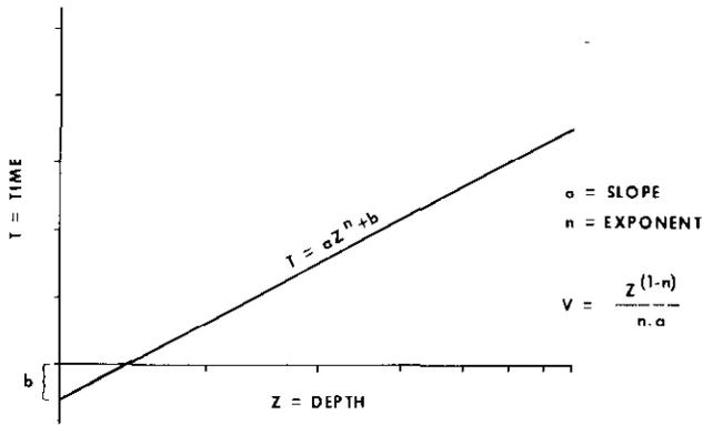
Fig. 15. Time-depth and velocity-depth relationship (Acheson, 1963).
