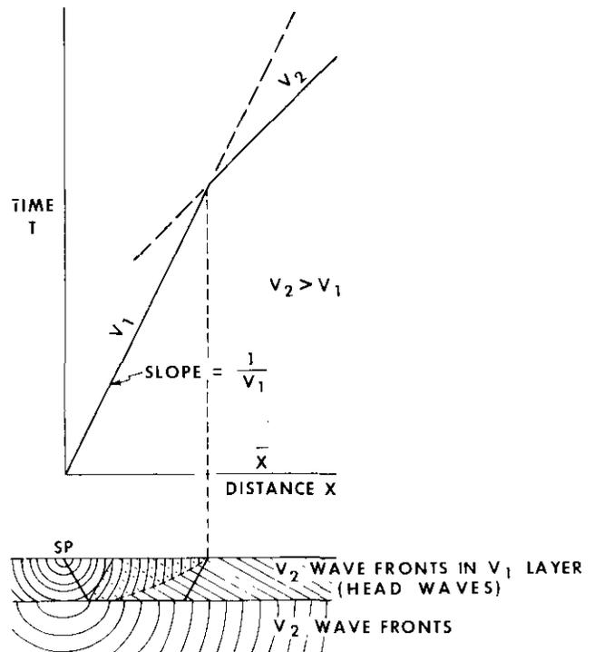
Fig. 4. Schematic wave fronts and time-distance curves.
