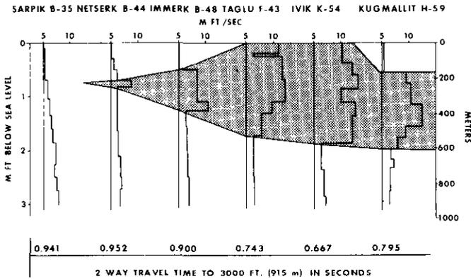
Fig. 3. Schematic section of permafrost changes across the Mackenzie Delta.
