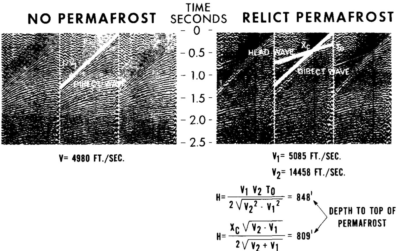
Fig. 5. Permafrost detection by refraction.
