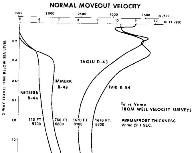
Fig. 16. Same curves as in Figure 8, showing permafrost thickness and  $V_{NMO}$  at one second for each well.
