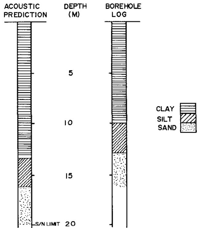
Fig. 10. Acoustic prediction versus borehole log.
