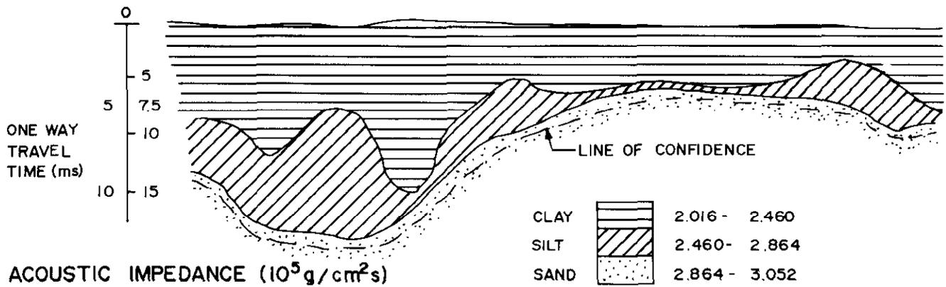
Fig. 11. Typical cross section of a river bed.
