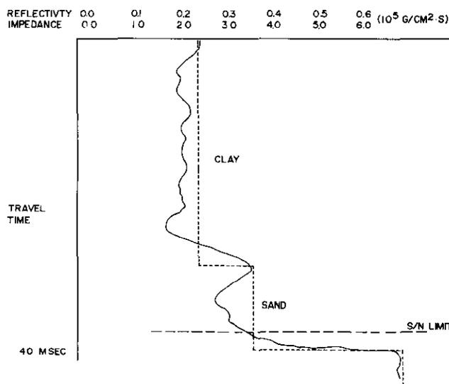
Fig. 4. Acoustic impedance as a function of travel time.
