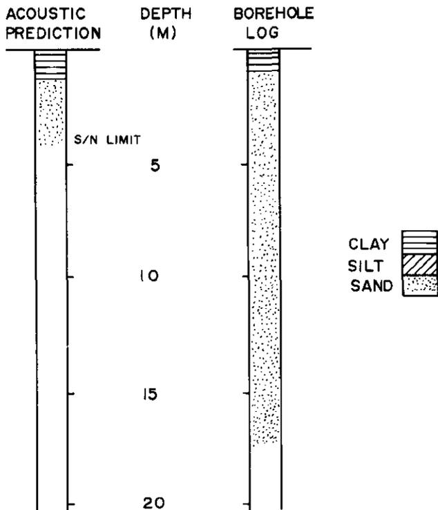
Fig. 9. Acoustic prediction versus borehole log.
