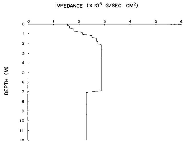
Fig. 3. Acoustic core - impedance versus depth.
