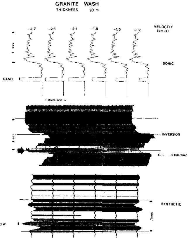
Fig. 17. Granite Wash sand of constant thickness of 20 m and velocity contrast with neighbouring carbonates and granites ranging from 1200 to 2700 m/s.
