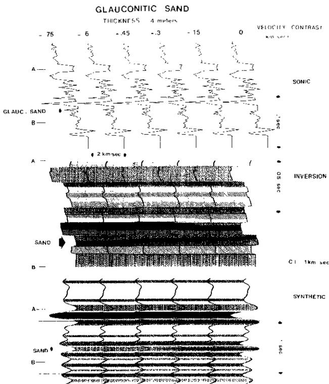
Fig. 9. Glauconitic sand of 4-m thickness and variable porosity. Velocity contrast after inversion in indicated zone between top and fourth inverted trace is 100 m/s, which suggests that 4-m-thick sand of velocity contrast with surrounding shales of 450 m/s should be detected.
