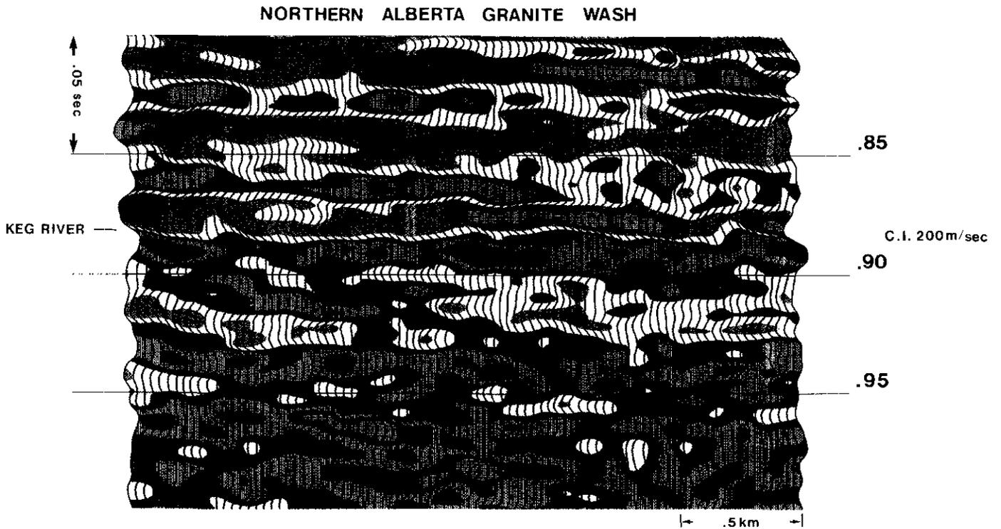
Fig. 18. An example of Granite Wash sand anomaly on inversion section (pale yellow). Zone indicated by the arrow is the likely location of Granite Wash at .90 s.
