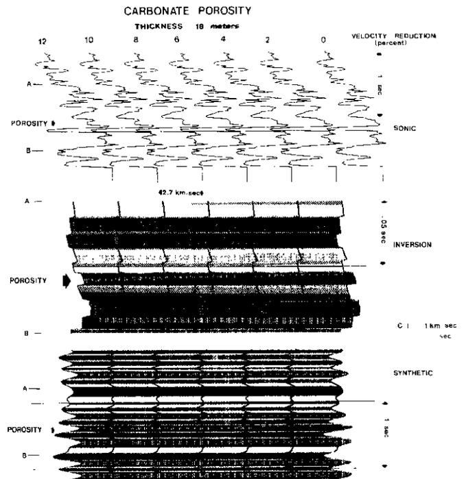
Fig. 13. Carbonate porosity near the top of Slave Point, thickness constant at 18 m and velocity contrast increases from 0 to 12%, which corresponds to porosity of 4 to 10% for water-filled carbonates with aspect ratio of .05 (Kuster and Toksoz, 1974). Difference in inversion velocity exceeds 100 m/s when contrast is 6%.
