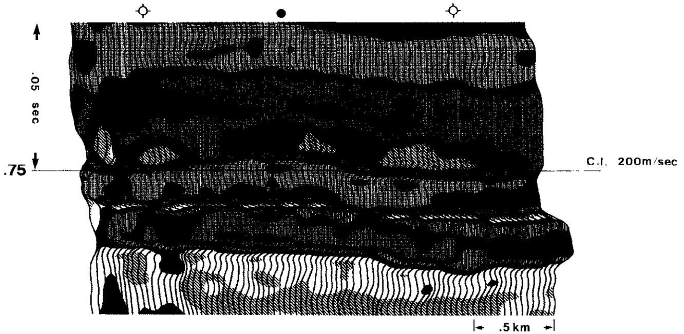
Fig. 11. Real data example where 3-m-thick porous oil-bearing sand is identified by lower velocity (red zones) at .75 s.
