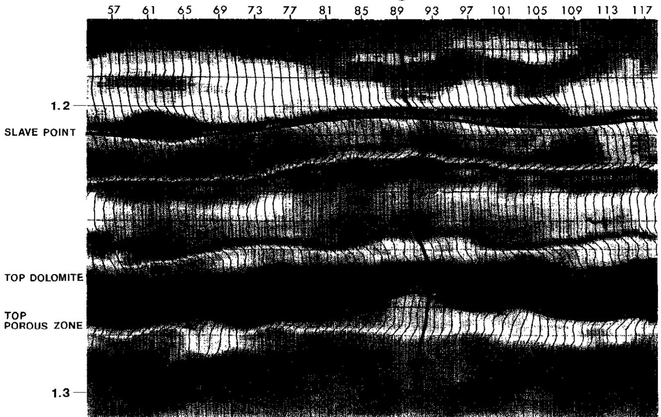
Fig. 14. An example of Keg River reef anomaly on inversion section. Porous zone is shown by thicker low-velocity zone (light blue) under Slave Point high (dark blue). |← .5 km →|
