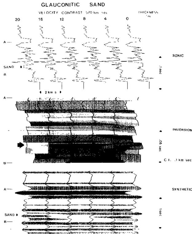
Fig. 8. Glauconitic sand with velocity contrast 570 km/s with neighbouring shales and of varying thickness. The sand is detectable when 4 m thick.
