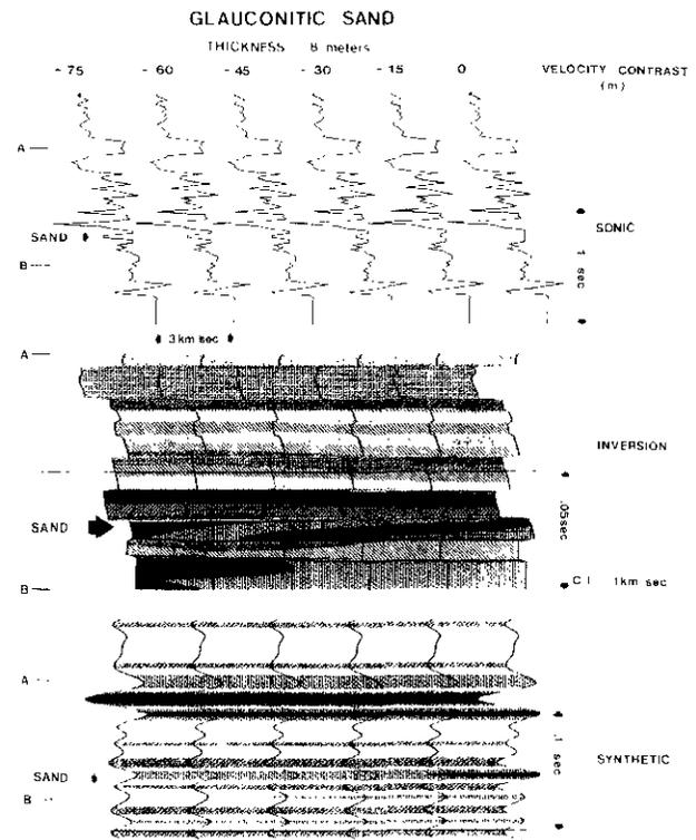
Fig. 10. Glauconitic sand of 8-m thickness and variable porosity. Velocity contrast after inversion in indicated zone between top and third inverted trace is 100 m/s, which suggests that 8-m-thick sand of velocity contrast with surrounding shales of 300 m/s could be detected.
