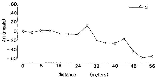
Fig. 4. Bouguer-corrected gravity anomaly data reduced to relative gravity with respect to station 0.
