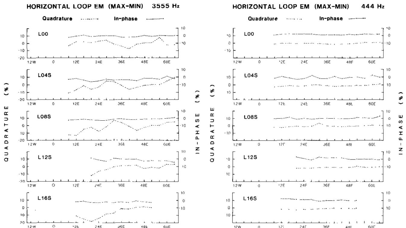
Fig. 11. Horizontal-loop (Max-Min II) electromagnetic profiles showing in-phase and quadrature responses at a frequency of 3555 Hz and 444 Hz.
