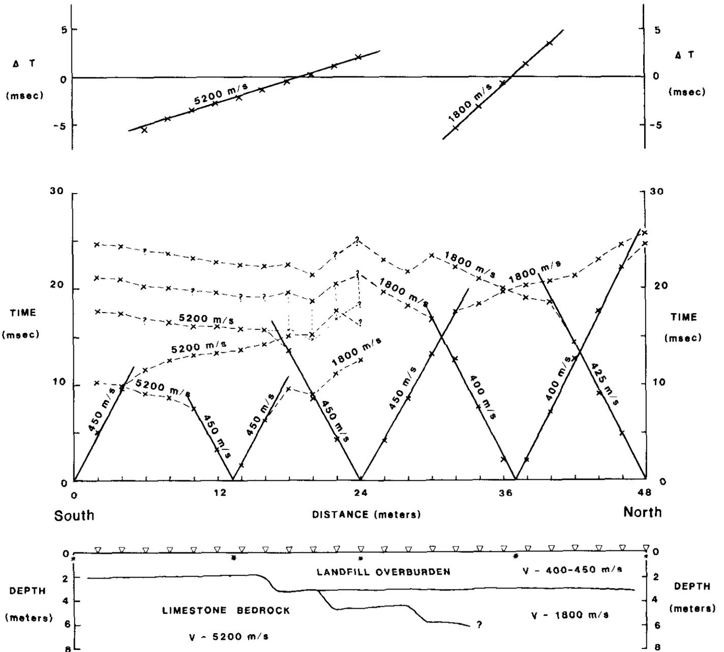
Fig. 5. Seismic refraction data and interpretation using intercept-time, delay-time and plus-minus techniques.
