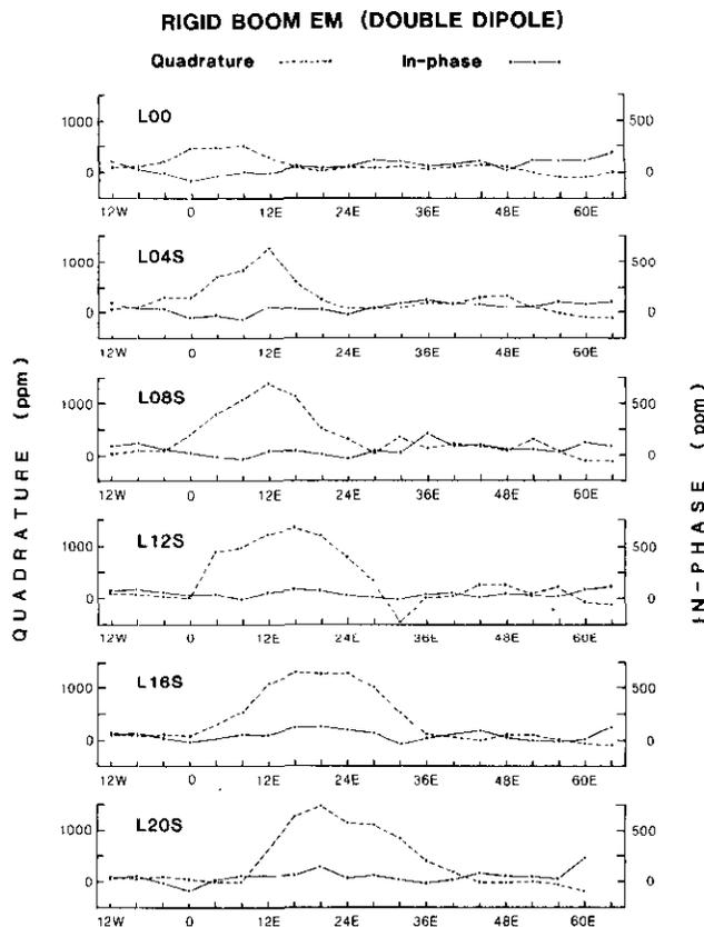
Fig. 10. Rigid-boom (Double-Dipole) electromagnetic profiles showing in-phase and quadrature responses. Note difference in scale between in-phase and quadrature plots.
