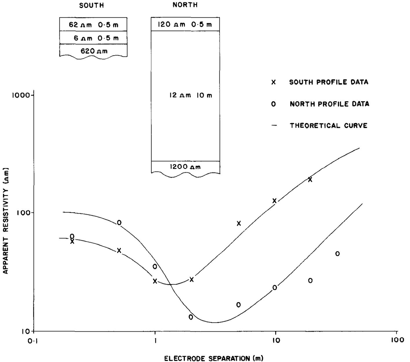
Fig. 3. DC resistivity sounding data and interpreted sections using three-layer curve-matching techniques from Elliot (1974).
