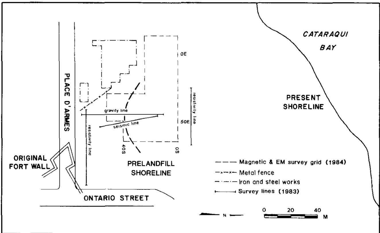
Fig. 2. Location map showing the positions of the resistivity, gravity and seismic surveys carried out in 1983, and the magnetic and electromagnetic survey grid used in 1984.
