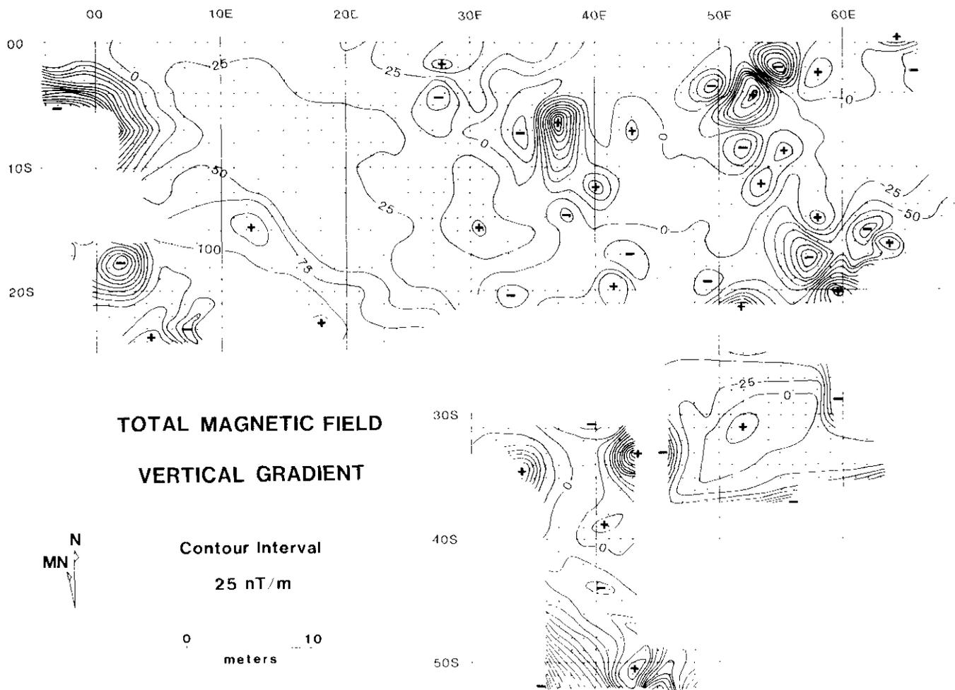
Fig. 9. Contoured total magnetic field; vertical gradient data over the archaeological site as in Figure 8.
