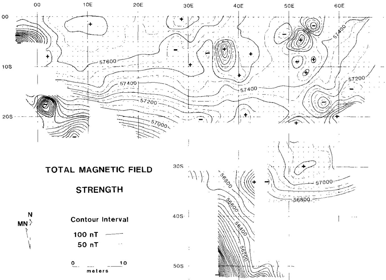
**Fig. 8.** Contoured total magnetic field strength data over the archaeological site. Each dot represents a measurement location.
