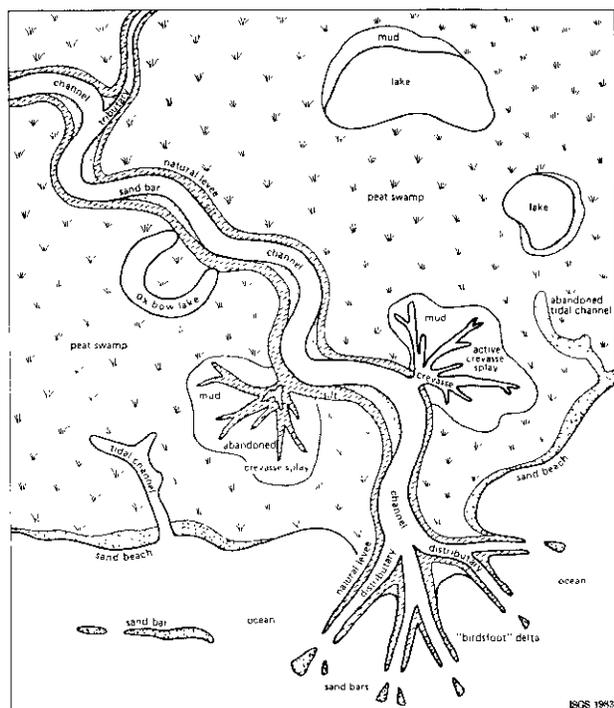
**Fig. 2.** Schematic diagram showing typical geologic features found near the mouths of large rivers in coastal plains.
