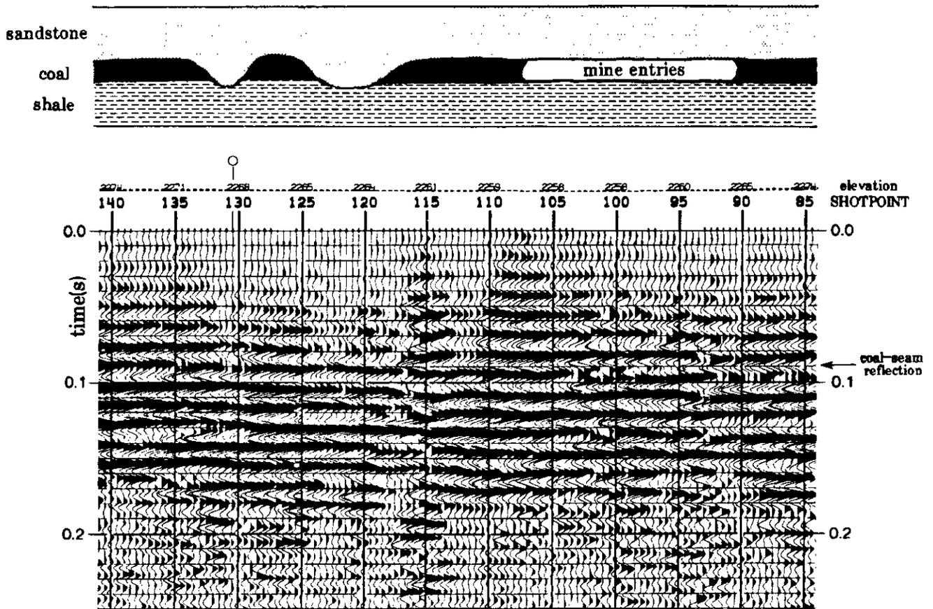
Fig. 6. Seismic section of Line 3.
