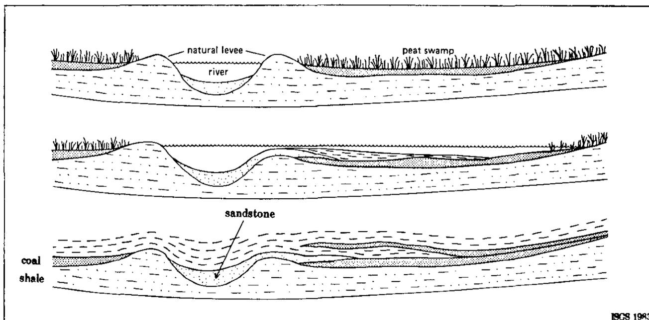
**Fig. 3.** Schematic diagram showing how periodic flooding produced splits in the seam near the river from overbank or crevasse-splay deposits.
