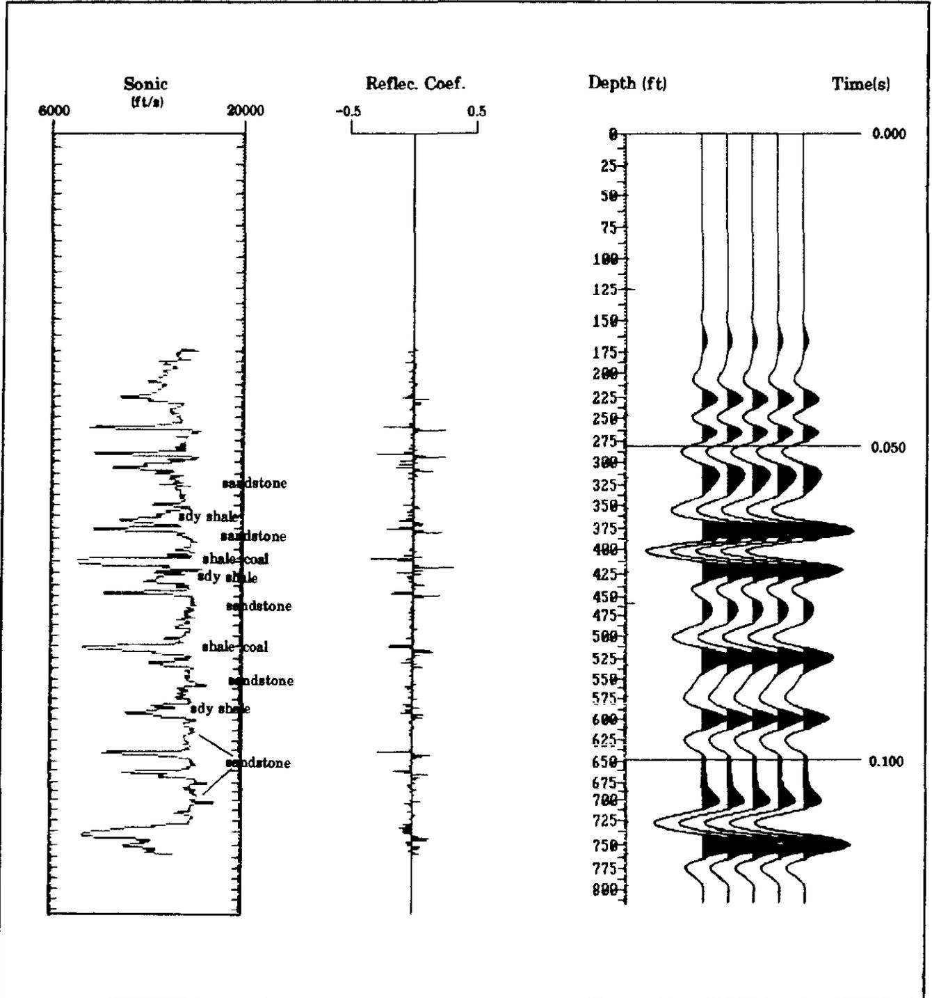
Fig. 4. Synthetic seismogram generated from a sonic log from a borehole near seismic Line 1, utilizing a 100-Hz Ricker wavelet. Key reflectors are indicated.
