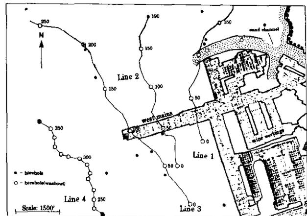
Fig. 1. Map of underground coal mine showing extent of mine workings.
