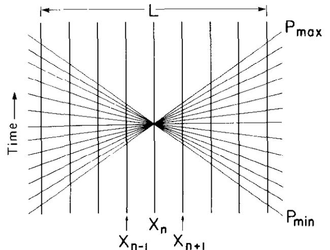
**Fig. 2.** Beam-forming diagram for multitrace dip and coherency analysis. Maximum and minimum dips are labelled  $p_{\max}$  and  $p_{\min}$ , respectively.  $x_n$  is the centre trace of an  $L$ -trace wide aperture. The dimensions of dip are given in either  $\text{km}^{-1}$  or  $\text{ms}/\text{trace}$ .
