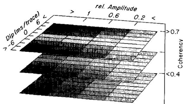
Fig. 5. (b) The colour ring (hue) represents automatically picked dip directions; lightness varies inversely with the 2-D smoothed local estimates of reflection strength, and saturation is controlled by local coherency estimates.
