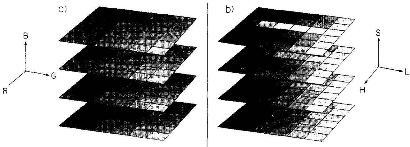
**Fig. 3.** Examples of multiattribute colour coding. Variations in the multiattribute  $M$  can be highlighted by defining its colour as a function of (a) red, green and blue (RGB) or (b) hue, lightness and saturation (HLS).
