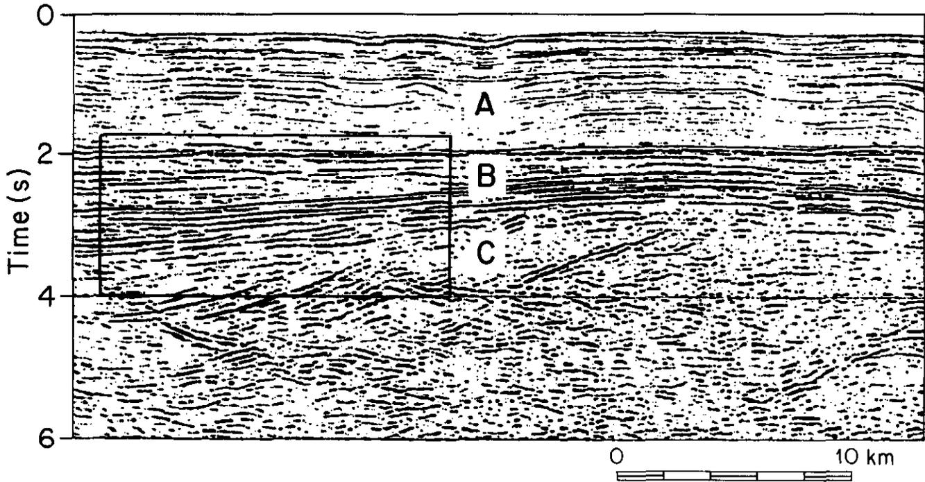
Fig. 4. Marine data example from the Midcontinent Rift (Lake Superior). The migrated section shows highly variable reflector dips and data quality. Multiattribute analysis of a 14-km portion of the data (insert) is shown in Figure 5.
