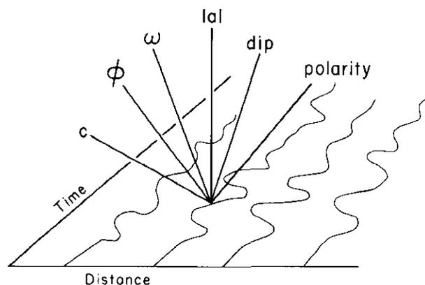
Fig. 1. Attributes of seismic data. Several attributes can be computed and assigned to each sample of the seismic wave field in the time-distance ( $t-x$ ) domain. Attributes used in this study are amplitude envelope (or reflection strength) ( $|a|$ ), coherency ( $c$ ) and dip. A multiattribute value  $M(x, t)$  is defined as the combination of two or more attributes, and colour coding is used for display purpose.
