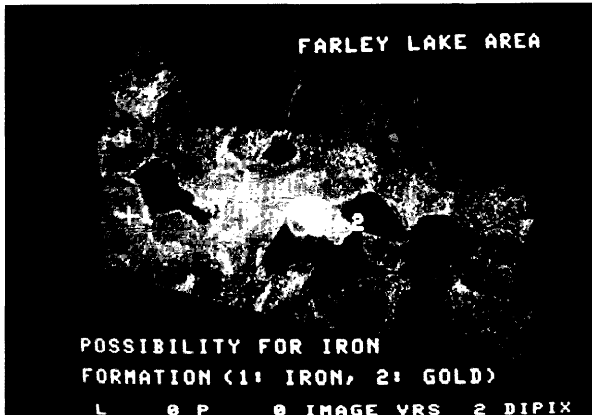
Fig. 12. (a) Possibility map for base metal displayed over a composite of bands 1 and 2 of the MEIS-II image over the test area. The blue hue (with contours) overlaid on the MEIS-II image represents the amplitude of the integrated fuzzy membership function towards the exploration target of base metal; (b) possibility map for iron formation displayed over a composite of bands 1 and 2 of the MEIS-II image over the test area. The blue hue on this image represents the fuzzy membership function, as above, but for the exploration target of iron formation.
