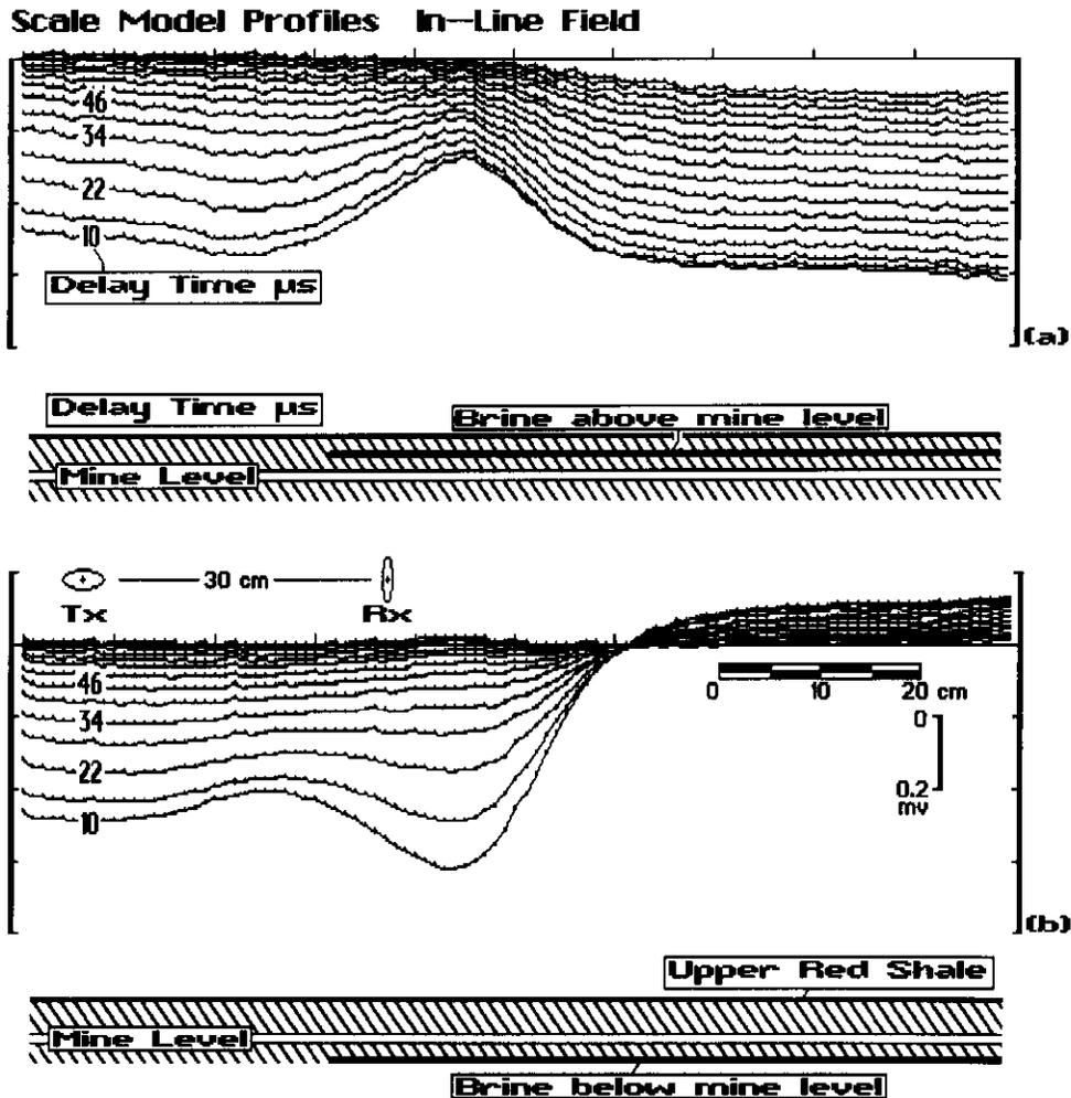
Fig. 3. (a) Scale-model transient electromagnetic profiles obtained with a model which placed a localized conductive layer above the mine room. The prominent anomaly is an edge effect due to this layer. (b) Profiles obtained when the localized layer was placed below the simulated mine room.
