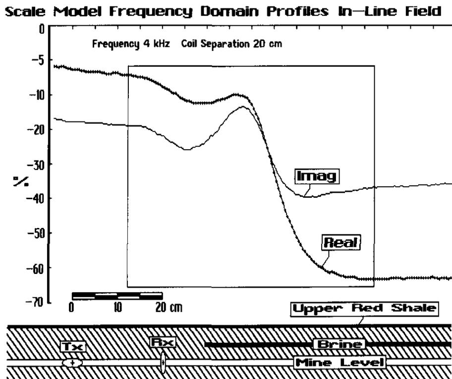
Fig. 6. Scale-model frequency-domain profiles of horizontal in-line field for a model which placed a localized sheet of conductor above the simulated mine room.
