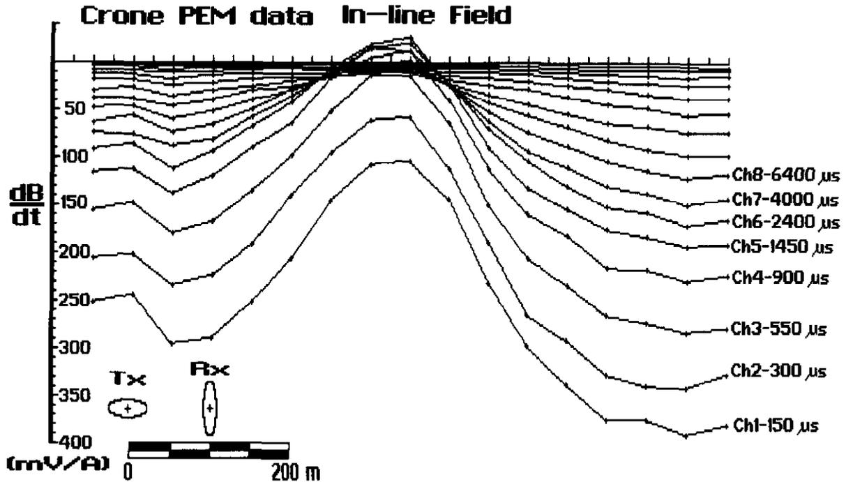
Fig. 1. Transient electromagnetic responses observed with the Crone PEM transient electromagnetic exploration system in a potash mine where water had been encountered in the mine operations.
