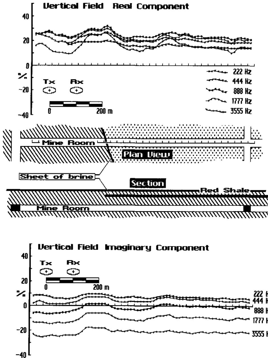
Fig. 7. Real and Imaginary component profiles of the vertical field component detected by a Max-Min frequency-domain electromagnetic survey along the traverse covered by the PEM survey in Figure 1. The lack of response to the horizontal sheet conductor is notable.
