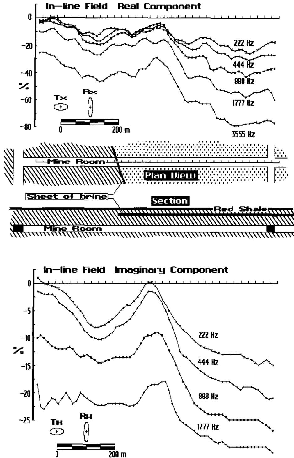
Fig. 5. Real and Imaginary component profiles of the in-line horizontal field detected by a Max-Min frequency-domain electromagnetic survey along the traverse covered by the PEM survey in Figure 1.
