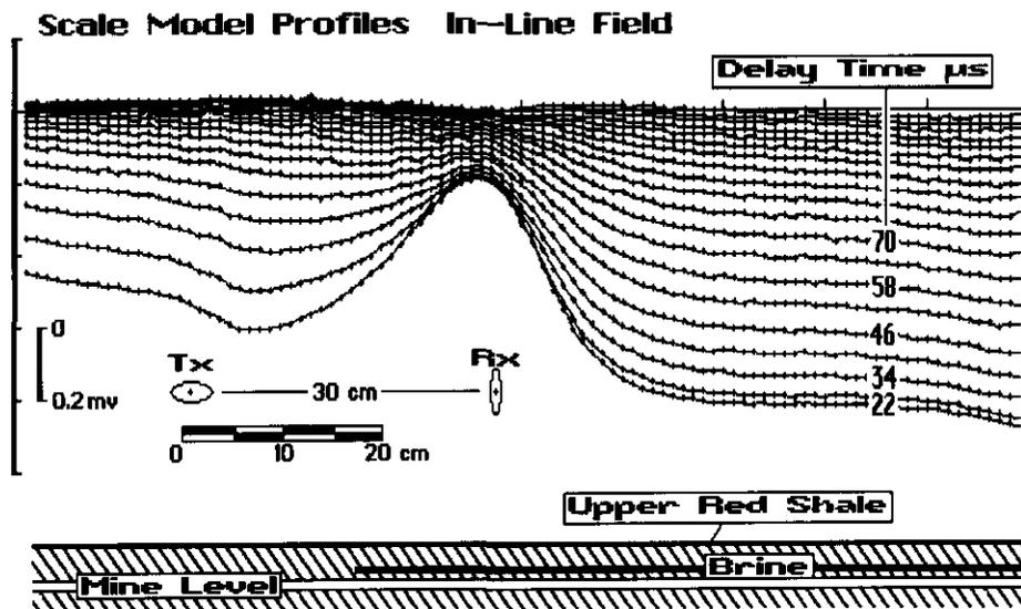
Fig. 4. Scale-model profiles obtained when the localized sheet of conductor was placed closer to the simulated mine room.
