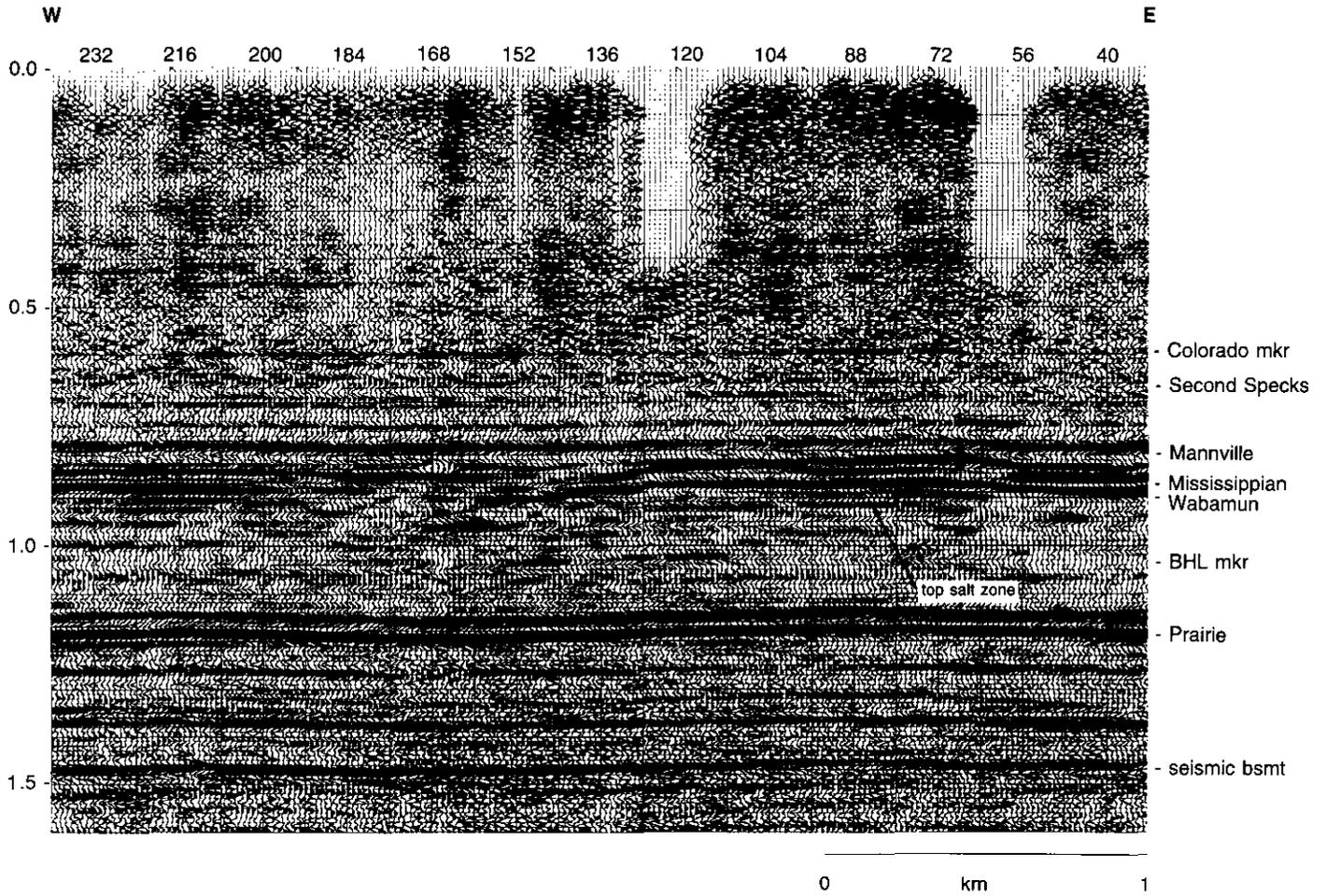
**Fig. 10.** Seismic line SL-1 (see Figure 2) crossing the isolated remnant of Wabamun salt displayed in Figures 4 and 9. The 6-20 well ties the seismic line at trace 104. These reverse-polarity 12-fold unmigrated data were acquired with the following parameters: single 0.5-kg dynamite charges at 18 m; a 33.5-m group interval; a 134-m shot interval; 96-trace split spreads (33.5 m – 1608 m) and a 2-ms sample rate.
