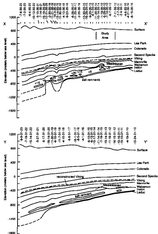
**Fig. 3.** West-east geologic profiles through the Stettler region illustrating the discontinuous nature of the Wabamun Group salts. The maximum known net thickness of rock salt in the Stettler area is approximately 40 m (Anderson and Brown, 1991b, 1992).
