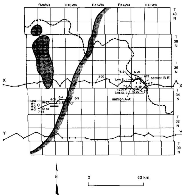
**Fig. 2.** Map of the Stettler region showing the margins of the Leduc reef complexes (solid lines) and the Wabamun subcrop edge (dashed line). The Sullivan Lake area (T34-35, R12-14W4), the approximate locations of the example seismic lines, and locations of the wells incorporated into Figures 5, 8 and 9, are also shown.
