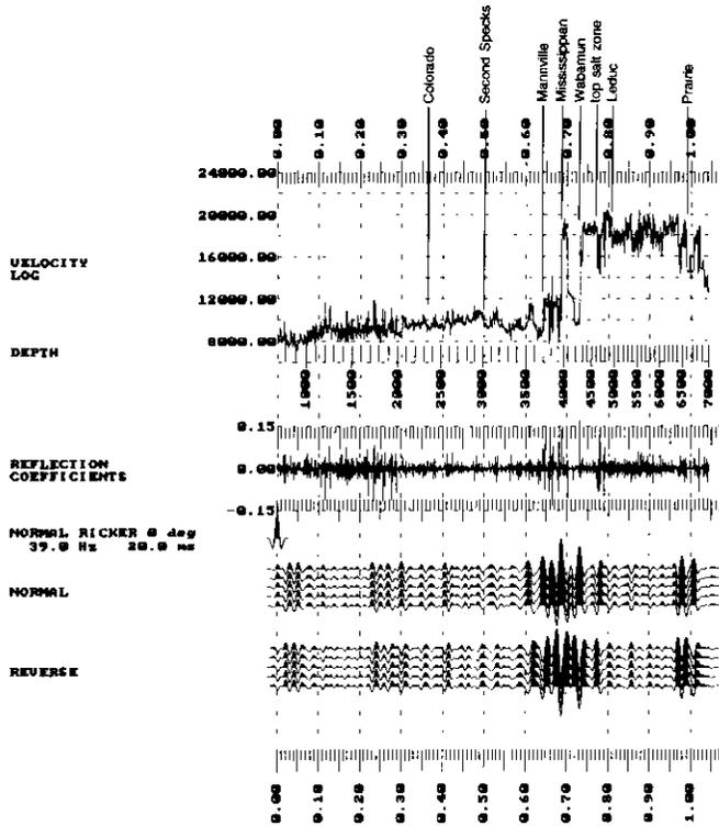
Fig. 8. Synthetic seismogram for the 2-20-35-16W4 well (Figure 2). This well encountered about 12 m (net) of Wabamun rock salt.
