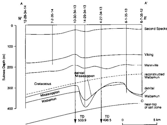
**Fig. 5.** Geologic section A-A'. Well locations are highlighted on Figure 2.
