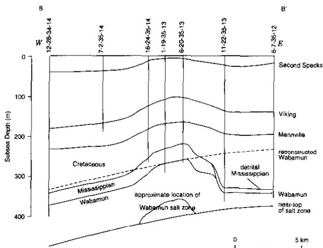
Fig. 9. Geologic section B-B'. Well locations are highlighted on Figure 2.
