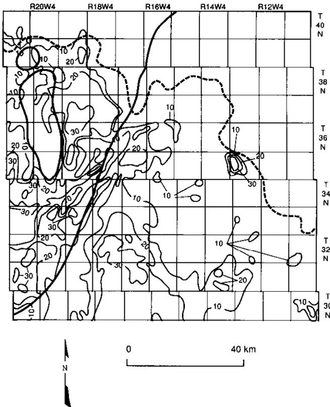
**Fig. 4.** Contour map (metres) of the area of Figure 2 depicting the interpreted present-day net thickness of the Wabamun rock salt in the Stettler region (modified after Anderson and Brown, 1991b). The salt remnant in T35, R13W4 is crossed by section B-B' and line SL-1 (Figure 2).
