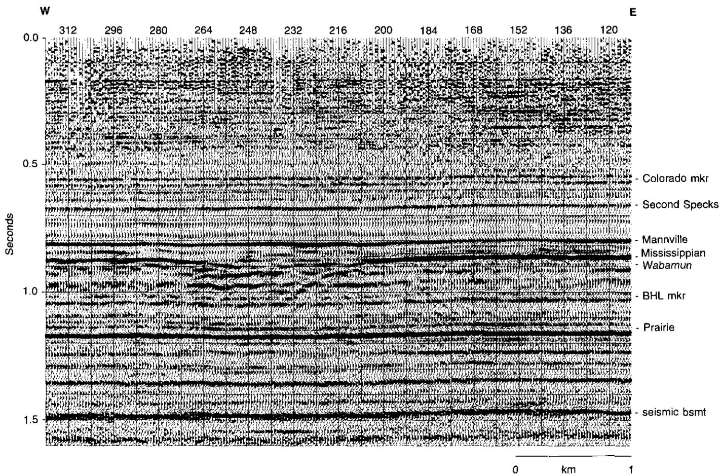
Fig. 6. Seismic line SL-3 (see Figure 2) crossing the Paleozoic channel displayed in Figure 5. Well 14-29 ties this seismic line at trace 248. These normal-polarity 24-fold unmigrated data were acquired with the following parameters: single 0.5-kg dynamite charges at 18 m; a 50-m group interval; a 100-m shot interval; 96-trace split spreads (50 m – 2400 m) and a 2-ms sample rate.
