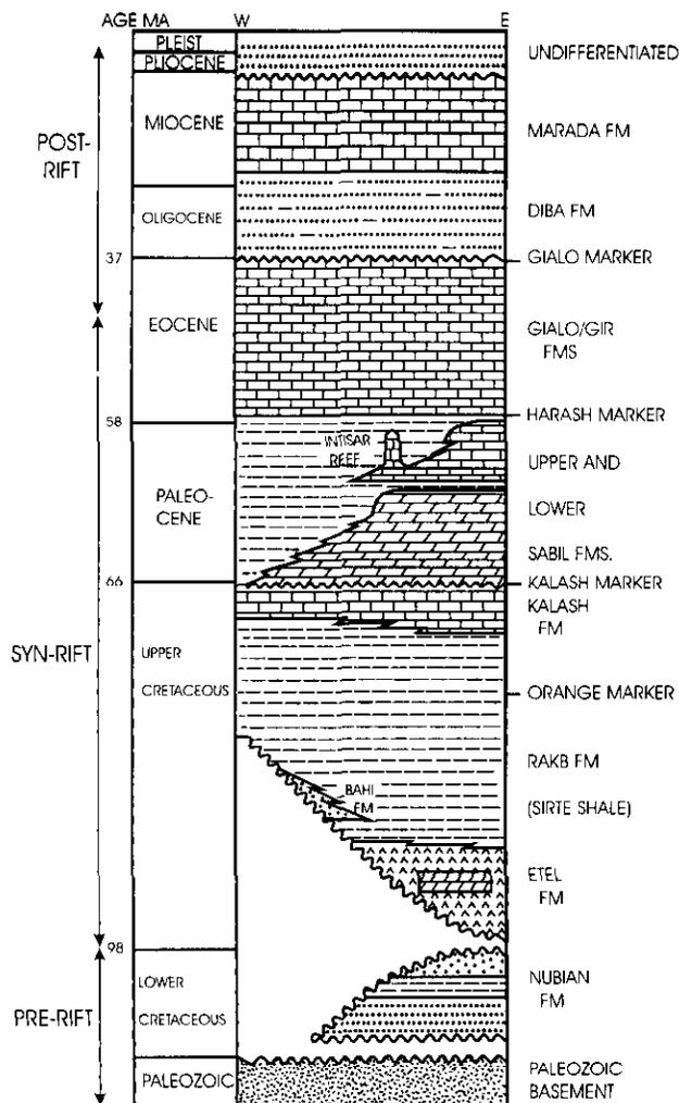
Fig. 2. Generalized stratigraphic column for the study area. The lower part of the Rakb Fm and the Etel Fm are not present on the Zelten Platform. No wells in the area have penetrated units older than the Orange horizon in the Agedabia Trough in the immediate area, so the deep geology is extrapolated from further away.
