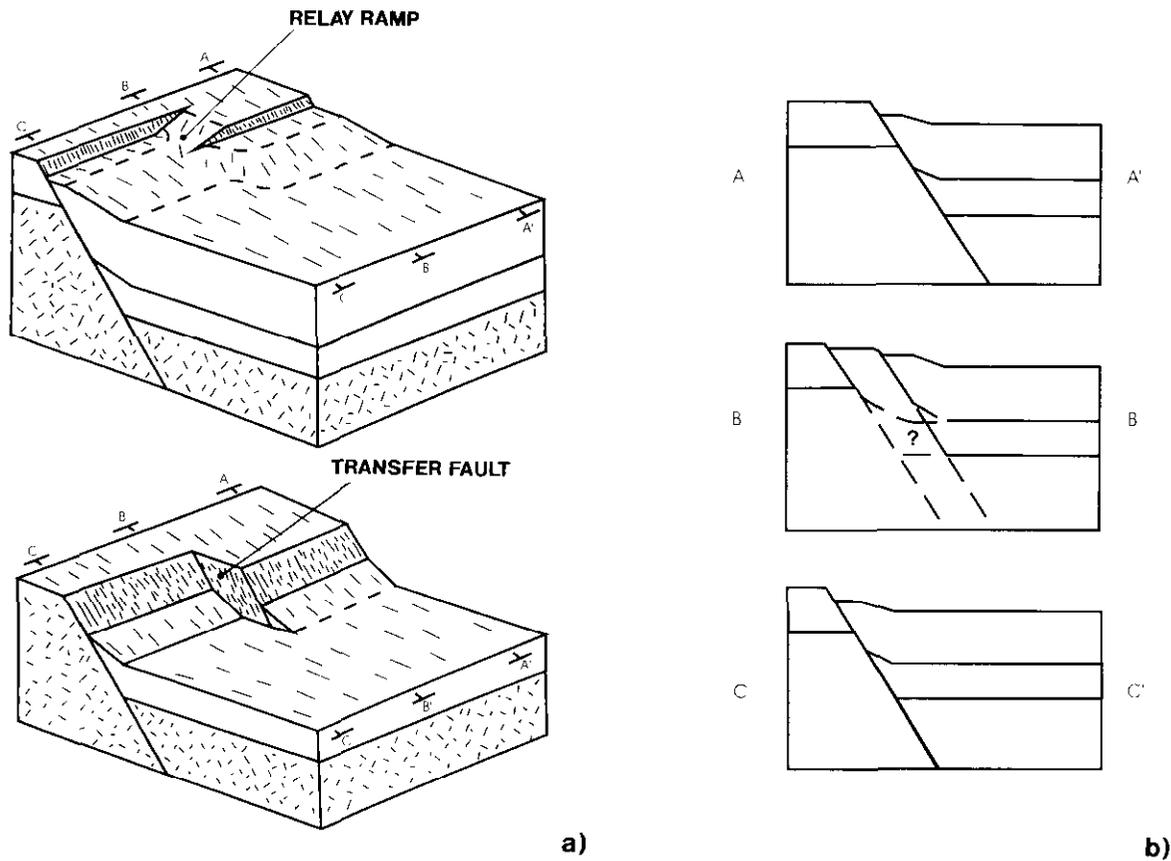
**Fig. 6.** Diagrammatic views of (a) and 'seismic' sections across (b) a normal fault and transfer zone. Section B, which runs above the transfer zone, will be contaminated with out of the plane energy and will be difficult to interpret. Note how the transfer zone changes in style with depth and how the compaction monoclines and relay structures interact.
