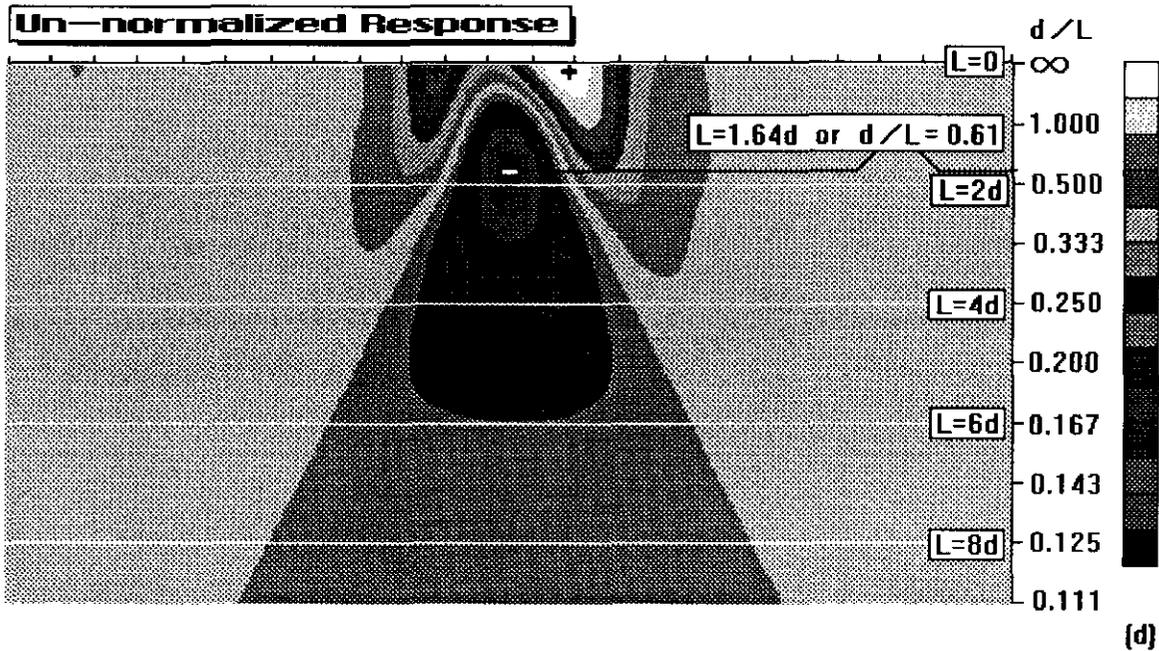
Fig. 1. (Cont'd) (c) Normalized theoretical response to a horizontal coplanar coil system of a thin perfectly conducting tabular conductor dipping at  $80^\circ$  in map form as a function of depth-to-separation ratio. (d) Absolute response of the same conductor showing the focussing of the response for a depth-to-separation ratio of 0.61.
