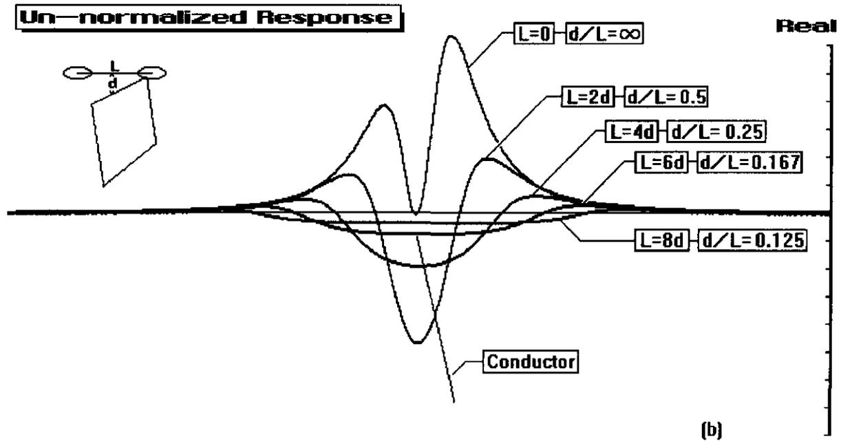
**Fig. 1. (a)** Normalized theoretical response to a horizontal coplanar coil system of a thin perfectly conducting tabular conductor dipping at  $80^\circ$ . **(b)** Absolute response of the same conductor (NB: the vertical scale is arbitrary, as the only intention is to demonstrate the relative magnitudes of the absolute responses).
