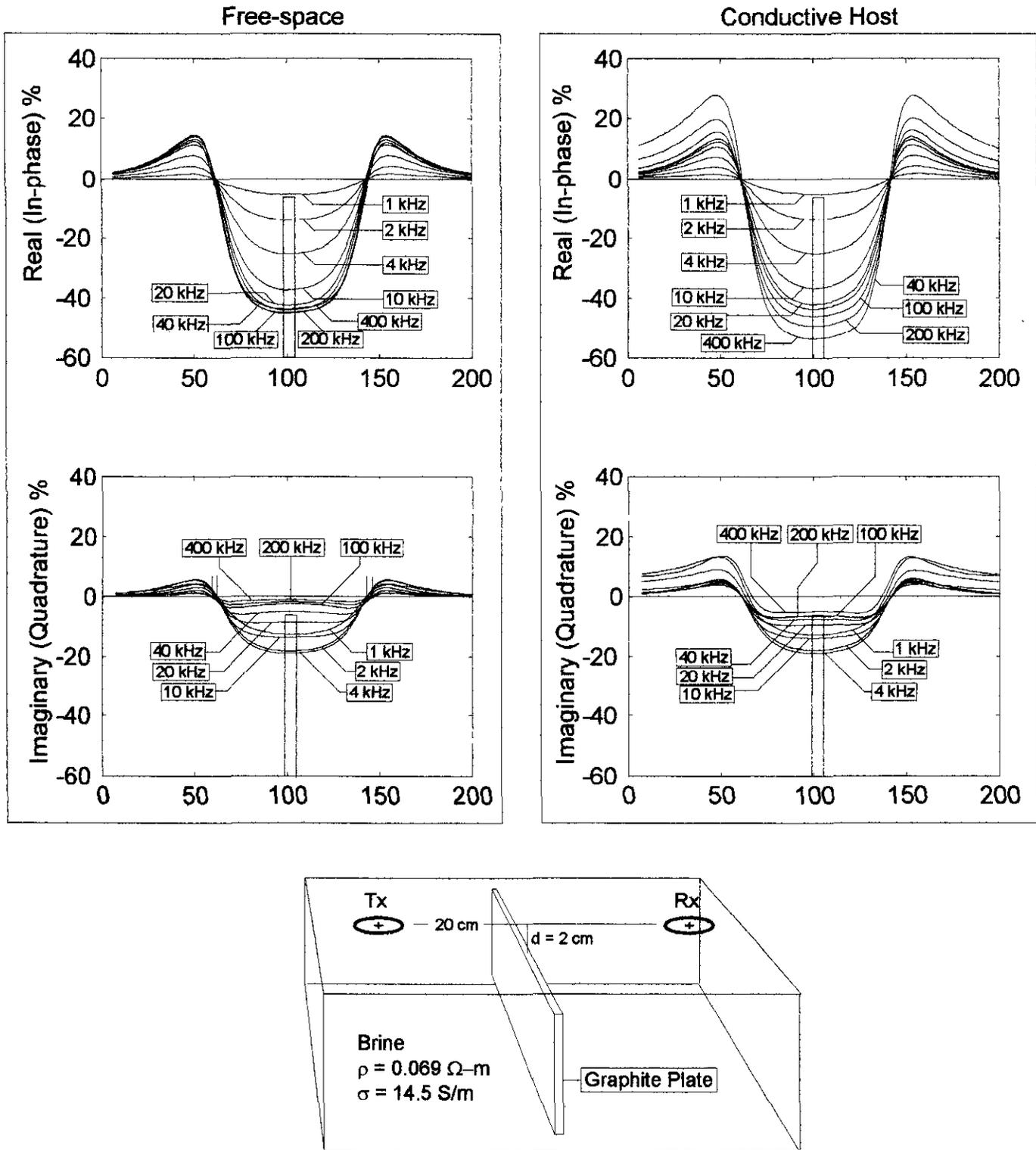
Fig. 1. Responses obtained with separated horizontal coplanar coils at a separation of 20 cm over a graphite slab target (dimensions 1 m x 0.3 m x 0.013 m) located at a depth of 2 cm first in a free-space host and then in a host of 14.5 S/m conductivity for a range of frequencies from 1 kHz to 400 kHz.
