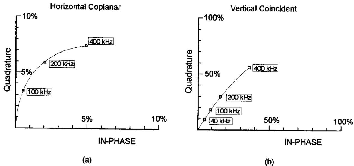
Fig. 6. Complex space plots of the response of the conductive host alone as detected by the coils in the separated horizontal coplanar configuration (a) and then in the vertical coincident configuration (b) for a range of frequencies and a depth of 2 cm.
