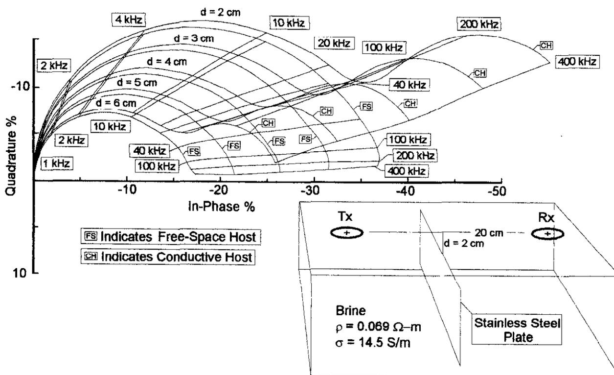
**Fig. 3.** Complex space plots of peak response obtained over a stainless steel target located at depths ranging from 2 to 5 cm and a frequency range from 1 kHz to 400 kHz using separated horizontal coplanar coils at a separation of 20 cm. The magnitudes in the main dispersion are too small indicating that possibly the magnetic permeability of the steel was affecting the response. These responses can not be used in quantitative interpretation of full scale field data.
