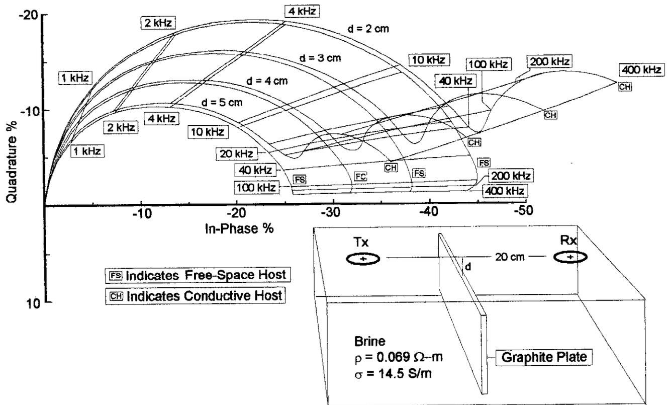
Fig. 2. Complex space plots of peak response obtained over a graphite slab target located at depths ranging from 2 to 5 cm and a frequency range from 1 kHz to 400 kHz using separated horizontal coplanar coils at a separation of 20 cm. The free-space host case and the conductive host case are superimposed for ease of comparison.
