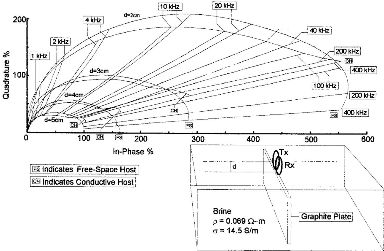
Fig. 5. Complex space plots of peak response obtained over a graphite slab target located at depths ranging from 2 to 5 cm and a frequency range from 1 kHz to 400 kHz using vertical coincident coils. The free-space host case and the conductive host case are superimposed for ease of comparison. The plotting scales of Figures 2 and 5 should be noted.
