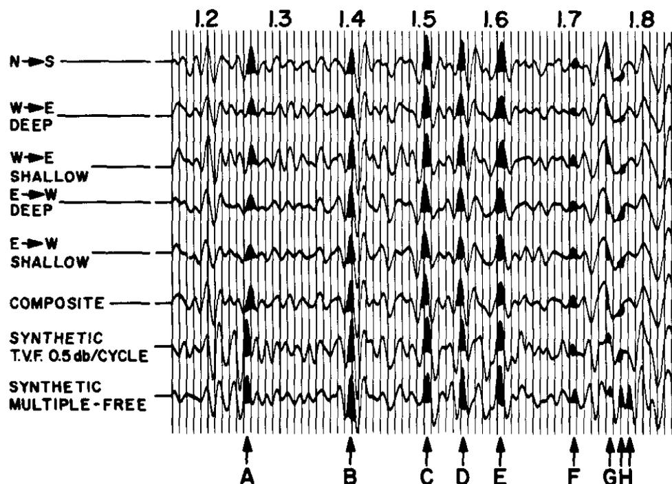
FIGURE 9. Test shots — T.A.R., deghost, Pie Slice deconvolution.
