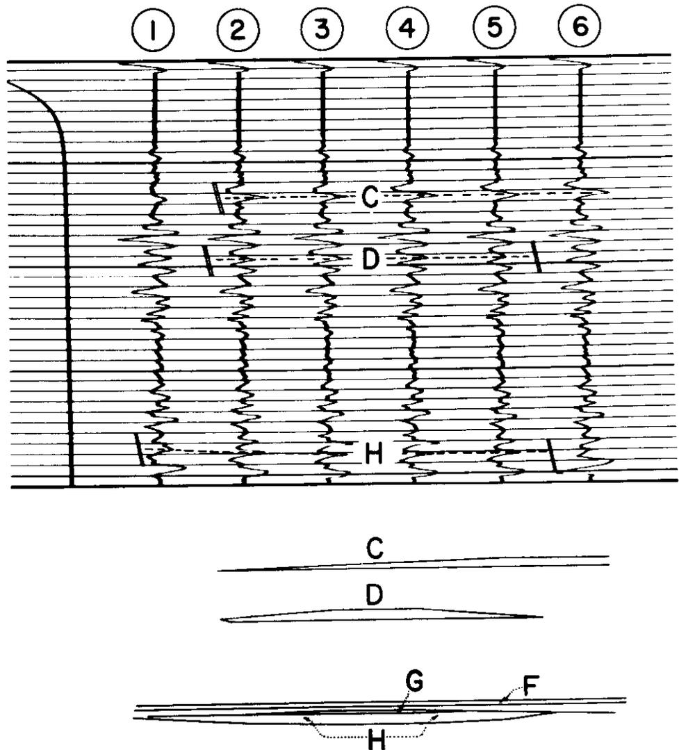
FIGURE 1. Synthetic seismogram — stratigraphic trap model.
