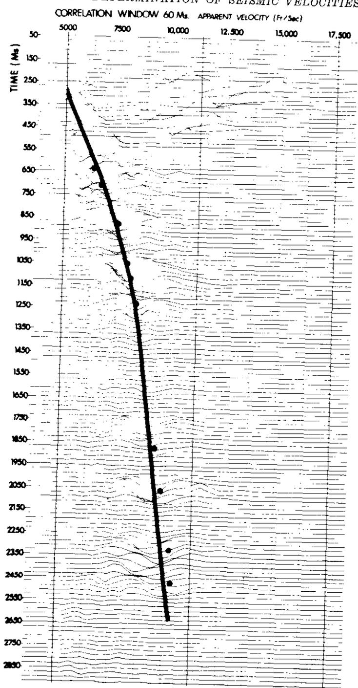
FIG. 6—Example of statistically normalized cross correlation as a coherence measure. A time gate of 60ms. with a 20ms. increment was used. At each time, a sweep of velocities from 5,000 ft/sec. to 20,000 ft/sec. in 50 ft/sec. increments was performed. The time-velocity axes are indicated. The input record was the same as in the previous examples.
