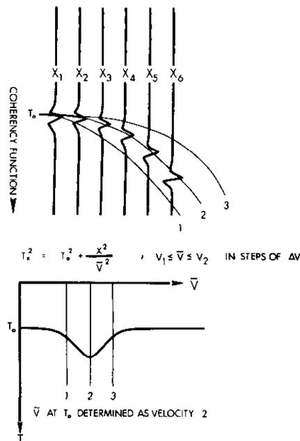
FIG. 3—Principle of computerized velocity analysis.
