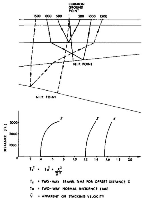
FIG. 2—Common depth point model for dipping layers.
