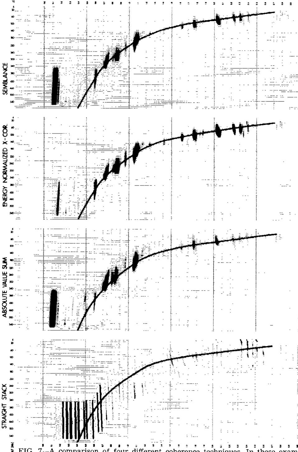
FIG. 7—A comparison of four different coherence techniques. In these examples, the coherency values were calculated at a constant delta-T search. Record time in seconds is indicated along the other axis. The input record was the same as in the previous examples.
