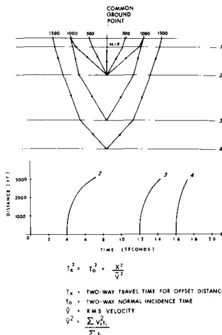
FIG. 1—Common depth point model for horizontal layering.
