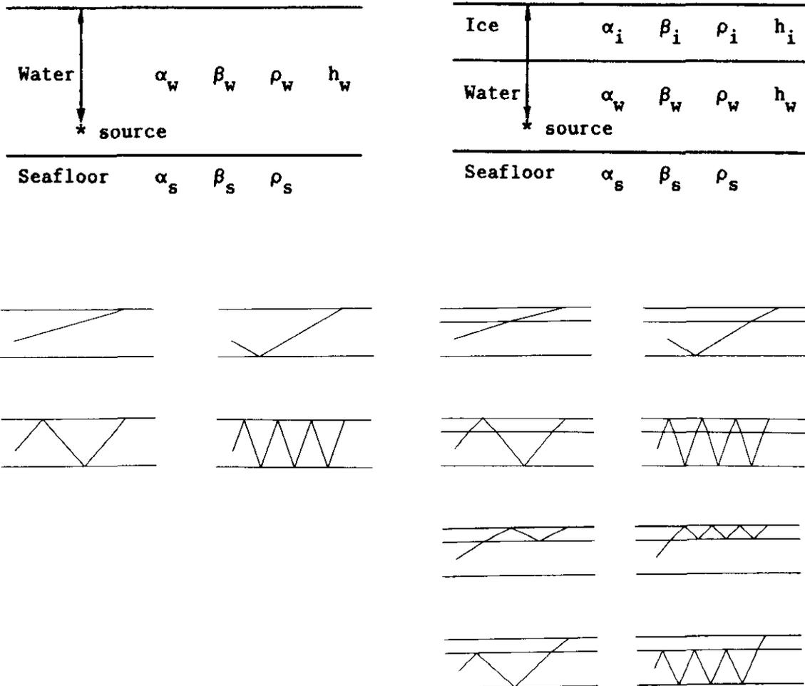
**Fig. 3.** The no-ice model and the ice model used to compute synthetic seismograms. Here  $\alpha, \beta, \rho$  and  $h$  are the  $P$ -velocity,  $S$ -velocity, density and thickness of the layer. For both models, the source is located in the water layer. The raypaths shown for the ice model are the typical raypaths of the four groups of waves: 1) primary waves, 2) ice-water multiples, 3) ice multiples and 4) water multiples.
