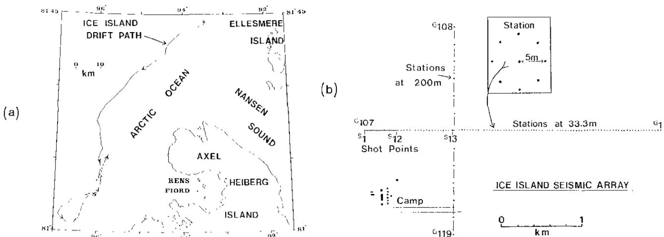
Fig. 1. (a) A map showing the drift path of the ice island during the summer of 1985 (after Cox, 1987). (b) Seismic array used to record the data in the ice island experiment. The main line has 107 stations. 13 shotpoints are located as shown with a source depth of about 110 m (after Cox, 1987).
