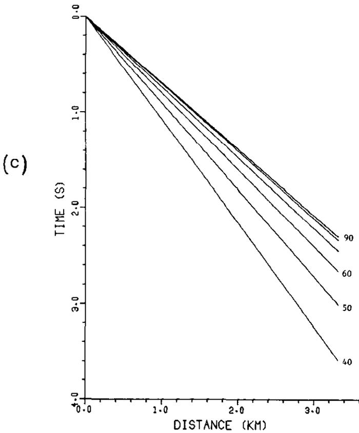
Fig. 11. (c) Amplitude cutoff lines for different critical angles at the seafloor for  $\alpha_w = 1.44$  km/s. The numbers are the critical angles in degrees.
