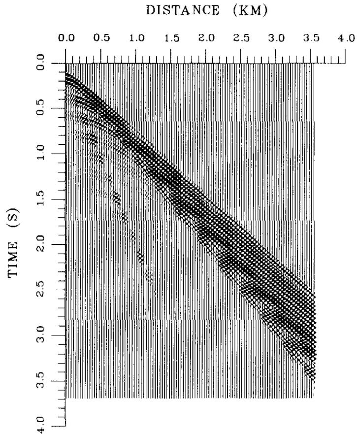
**Fig. 6.** Synthetic section for a no-ice model with a hard seafloor (case 1:  $\alpha_s = 4.0$  km/s,  $\beta_s = 2.0$  km/s,  $\sigma_s = 0.33$ ).
