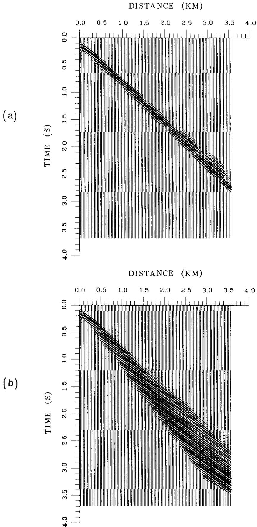
**Fig. 11.** (a) Synthetic section for an ice model with a soft seafloor (case 5:  $\alpha_s = 1.6$  km/s,  $\beta_s = 0.6$  km/s,  $\sigma_s = 0.42$ ); (b) (case 6:  $\alpha_s = 2.2$  km/s,  $\beta_s = 0.6$  km/s,  $\sigma_s = 0.46$ ).
