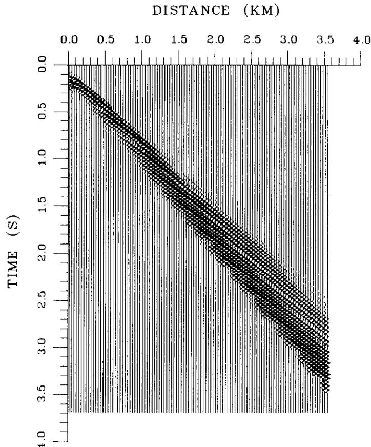
Fig. 10. Synthetic section for an ice model with a soft seafloor (case 4:  $\alpha_s = 2.0$  km/s,  $\beta_s = 0.6$  km/s,  $\sigma_s = 0.45$ ).
