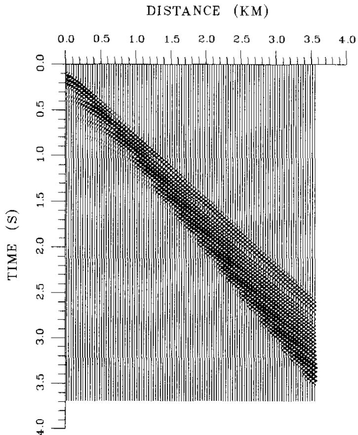
**Fig. 7.** Synthetic section for a no-ice model with a soft seafloor (case 2:  $\alpha_s = 2.0$  km/s,  $\beta_s = 0.6$  km/s,  $\sigma_s = 0.45$ ).
