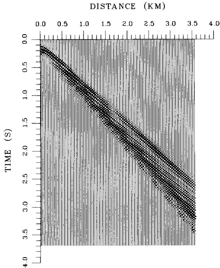
Fig. 9. Synthetic section for an ice model with a hard seafloor (case 3:  $\alpha_s = 4.0$  km/s,  $\beta_s = 2.0$  km/s,  $\sigma_s = 0.33$ ).
