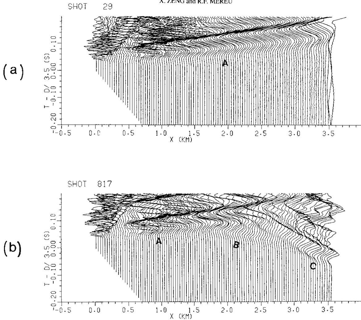
**Fig. 13.** (a) First-arrival data for shot 29. The main traveltim branch (A) is a *P*-wave branch from the ice layer with a velocity of 3.36 km/s. (b) First-arrival data for shot 817. There is an ice branch (A) with a velocity of 3.36 km/s and two sedimentary branches (B) and (C) with velocities 4.0 km/s and 5.3 km/s.
