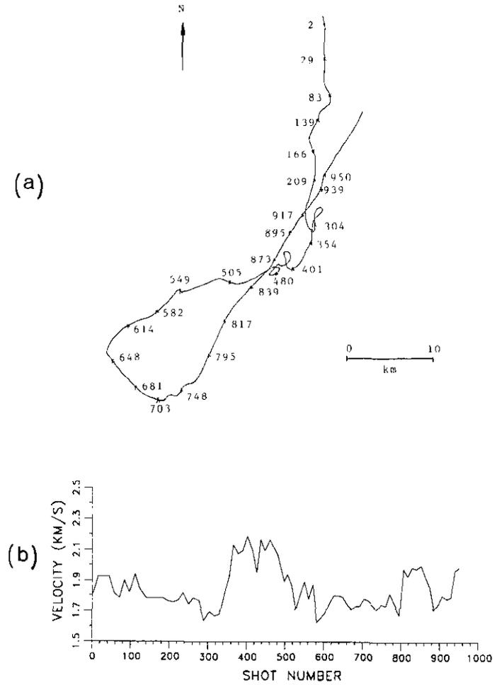
Fig. 12. (a) The locations of different shots along the drift path of the ice island. The numbers are the shot numbers. (b) Seafloor velocity profile along the drift path shown in Figure 12(a).
