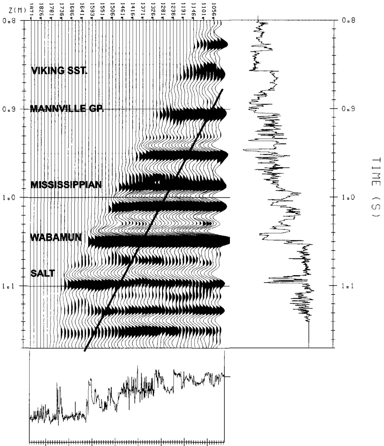
**Fig. 3c.** Waveshaped upgoing VSP wavefield (+TT) compared to impedance logs in time (constrained by corrected checkshots) and in depth (TVD, SRD = 900 m). The concept of inside corridor stacking is illustrated by the mute zone. Some geologic entities are identified.
